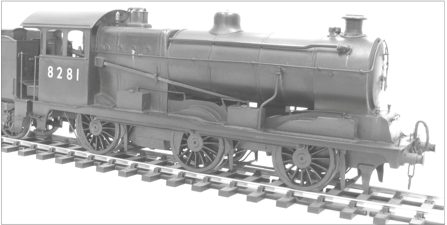
Detail View of Sandbox Operating Rods. Reverser Rod and its Support Bracket on Fire Box Side.
